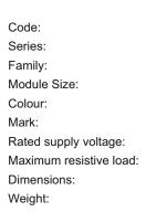
C5160 .01 CUBE Series Switches Two Module Frost White Norisys 230V 16A 55.6mm x 44.8mm x 34.3mm 37.1g
